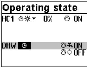
\* Activate editing mode for the control circuit. The operating mode is shown inverted on the display.
