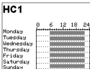
Turn the rotary switch to
