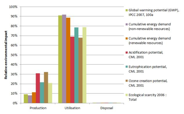
The relationship of the contributions made by the utilisation in comparison to those made by the production and disposal depends on the intensity of the utilisation (utilisation scenario).
