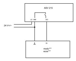
The MM terminal of the ASV 2<sup>\*\*</sup> to be connected must be connected to the ground of the ecos500 and the modu525.
